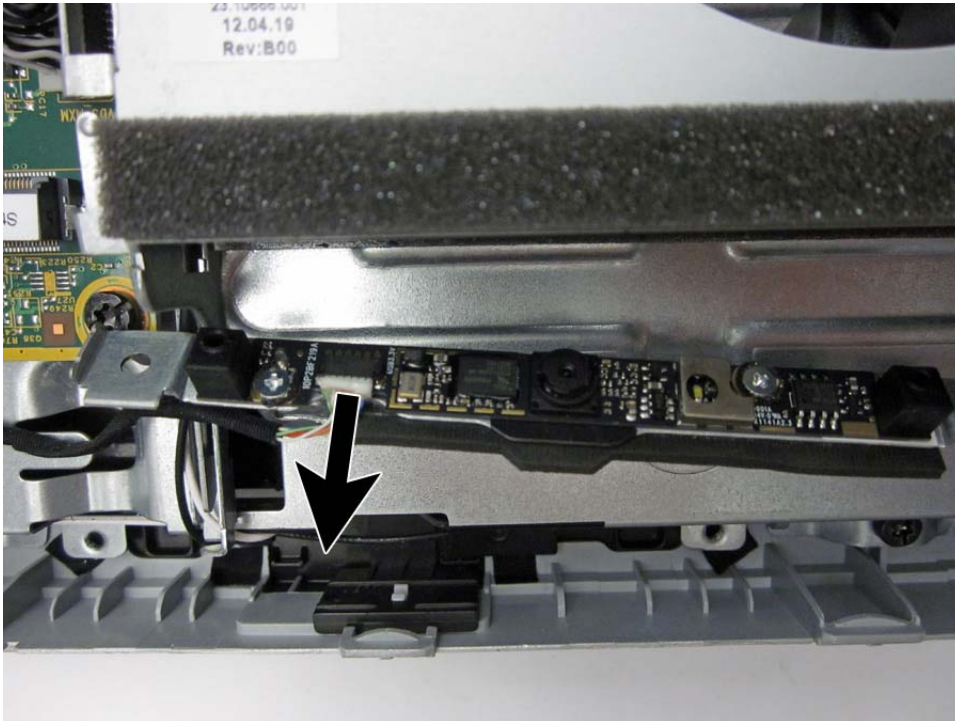
Figure 6-43 Disconnecting the webcam module cable
